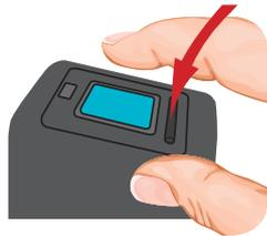
Without touching the sensor, position your finger so that the first joint rests on the ridge lock (shown by red arrow)
