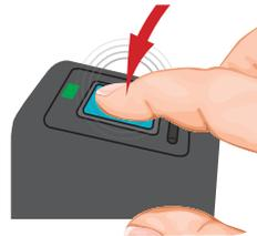
Using moderate pressure, place fingertip on sensor. The amber light will turn green while scanning.
